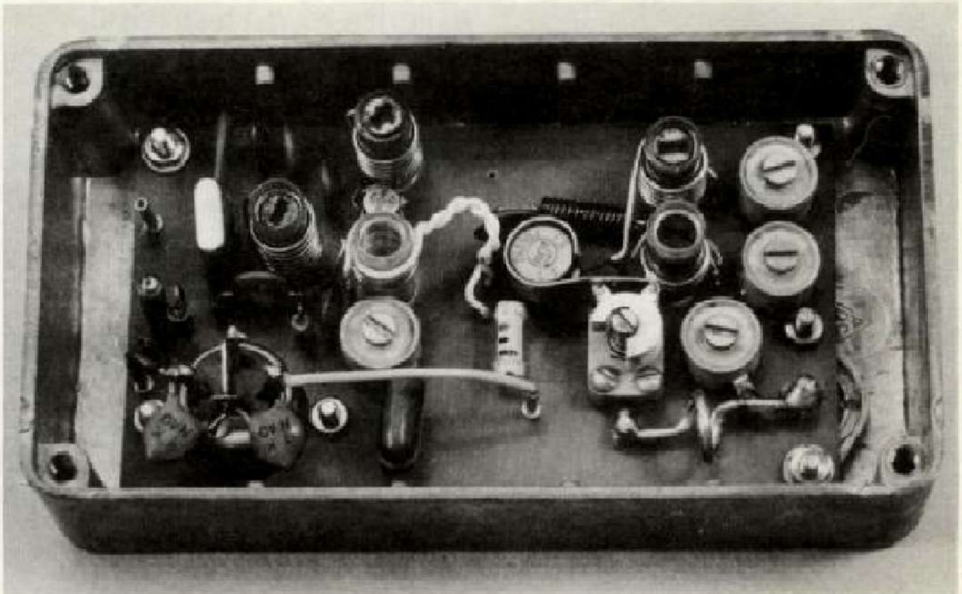
Fig.6.97. A 432 MHz 150mW exciter using a 2N3553 by a GM290 mounted into a standard diecast box. The circuit for this unit is shown in Fig.6.98.
