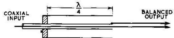
Fig.9.6. Coaxial sleeve balun.
